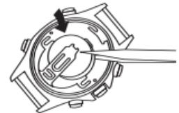
4. The battery type is a 3.0 Volt CR2032 Lithium Battery.
