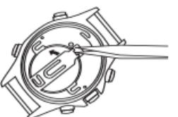
2. There is a protective label over the battery. This is required for insulation purposes and must be replaced when the new battery has been fitted
