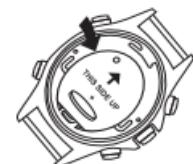
6. Replace the case back making sure that the battery is correctly fitted, that the rubber seal around the case back is seated properly, that the case back fits without interference and is the correct way up. If possible add some silicon grease or Vaseline to the rubber seal.
