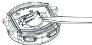
4. The battery type is a 3.0 Volt CR2032 Lithium Battery.
