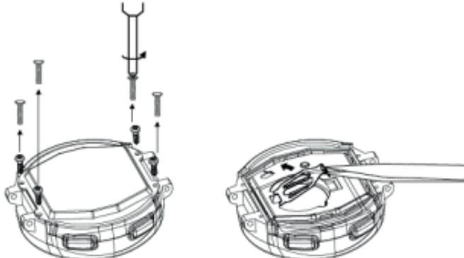
2. There is a protective label over the battery. This is required for insulation purposes and must be replaced when the new battery has been fitted
