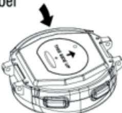
6. Replace the case back making sure that the battery is correctly fitted, that the rubber seal around the case back is seated properly, that the case back fits without interference and is the correct way up. If possible add some silicon grease or Vaseline to the rubber seal.
