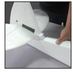
7 Insert the horizontal stabilizer and vertical stabilizer in place.
