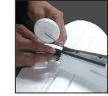
Install the servo horn of rudder with M2\*14 screw.
