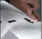
4 Fix the wing on fuselage with M6\*35 screw.
