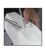
6 Install the front landing gear with PT M3\*6 screw.
