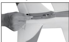
Insert one end of the Z-shapped pushrod into servo arm and aother end into the rudder servo horn.
