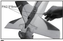
Secure the vertical stabilizer with PA2.5\*8mm screws.
