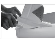
Apply glue to the elevator and install it on the fuselage.
