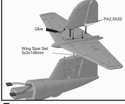
2 Use the carbon tube to connect rudder and elevator, fix them with screws and then glue them together.
