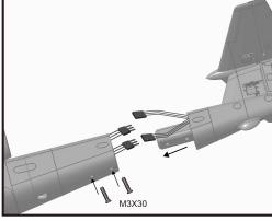
3 connect the rudder and elevator servos and fix the stabilizer into fuselage with screw.
