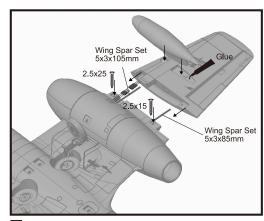
1 connect the aileron servos with wires. Insert the carbon tube into the main wing and connect the left and right wing to the main wing with this carbon tube. Use the screws to fix them. Fix the auxiliary fuel tank with glue.
