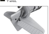
8 Fix the stabilizers with PA2.3\*20mm 9 Install elevator push rod as shown.
