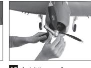
12 Install the propeller.
