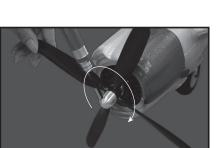
6 Install the propeller.
