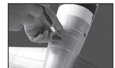
1 Install the horizontal stabilizer and vertical stabilizer. Secure the stabilizers with PA2.3X20 screw.
