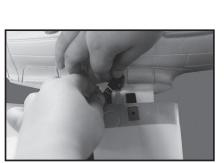
2 Connect the cables between aileron servo, flap servo and the LED indicators.
