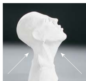
Arrows indicate undercuts.
