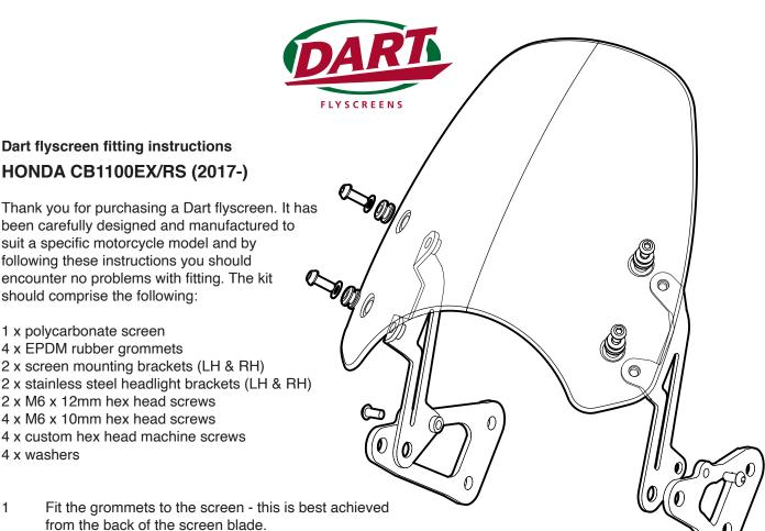
1 Fit the grommets to the screen - this is best achieved from the back of the screen blade.
