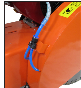
Double water pipe for cooling both side of blade
