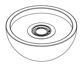
This is a freestanding decorative bio ethanol fireplace that is made for OUTDOOR USE ONLY. There must be minimum 2 m clearance above the firepit at all times and minimum 1.5 m clearance between the firepit and any flammable materials, including trees or shrubbery (check installation instructions for more details).
