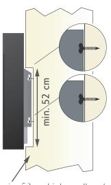
min. 52 cm high to allow for enough space around the firebox and the stainless steel container
