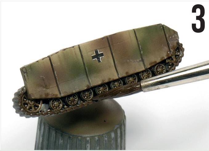
Apply the mixture of pigments and thinner on the tracks.
