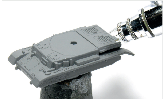
Airbrush couple of thin layers of the primer
