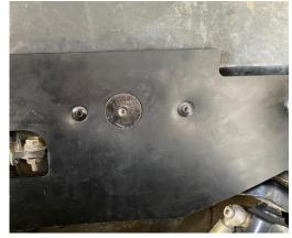
10. Slide the front most side of the debris shield behind the bed rib as shown. Adjust the Debris shield until adequate fitment is achieved and hand tighten the 10-24 screws in place.
