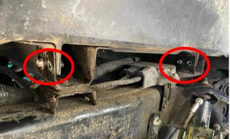
4. Loosely Secure 1 Rear Bed Frame Brackets W/ PEM in place utilizing 1/4 Flat Washer and 1 M6 Hex Head Bolt onto the left most bed support. Repeat on the right most bed support.
