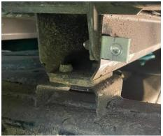
16. Feed the Rear Debris Shield Driver into the wheel well.
