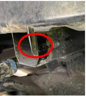
14. Loosely Secure 1 Rear Bed Frame Brackets W/ PEM in place utilizing 1/4 Flat Washer and 1 M6 Hex Head Bolt onto the left most bed support. Repeat on the right most bed support.
