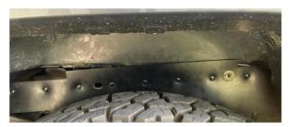
17. Secure each side of the debris shield in place with 1 10-24 Screw and 1 Fender Washer.
