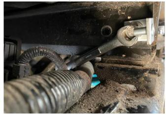
7. Rotate the Right most bracket up as shown and hand tighten the M6 Hex Bolt in place. This side is accessible from the bottom with a 10mm wrench.
