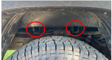
3. Remove the 2 front most bolts utilizing a 10mm socket or wrench.
