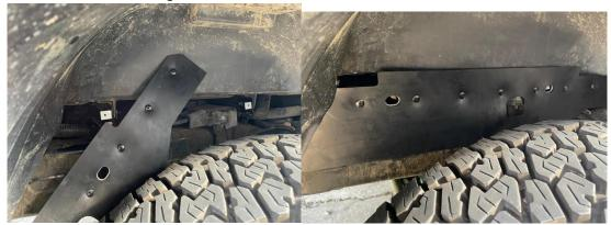
9. Secure each side of the debris shield in place with 1 10-24 Screw and 1 Fender Washer.
