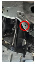
13. Secure the Front most end of the Front Debris Shield Passenger in place 1 Plastic Push Rivet **SHORT** and 1 Washer.
