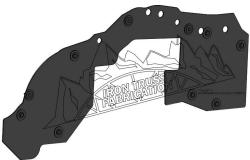
6. Secure the Front Debris Shield Passenger in place <u>UNDER</u> the OEM felt wheel well liner with 1 Plastic Push Rivet **LONG** and 1 Washer.
