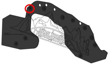
20. Secure the front most end of the Front Debris Shield Driver in place to the Vehicle Frame with 2 Plastic Push Rivets **SHORT** and 2 Washers.
