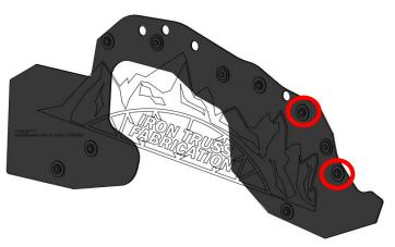
24. Secure the rear most end of the Front Debris Shield Driver in place to the Vehicle Frame with 1 Plastic Push Rivet **SHORT** and 1 Washer.
