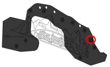
23. Secure the front most end of the Front Debris Shield Driver in place with 2 Plastic Push Rivets **SHORT** and 2 Washers.
