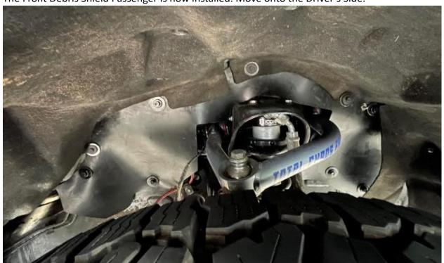
15. Remove the 4 Push Rivets Holding the OEM Felt Wheel Well liner to the body of the vehicle on the Driver's Side of the vehicle.
