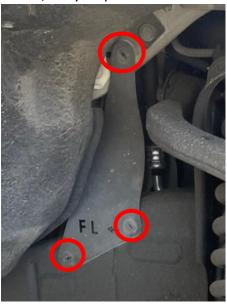
3. Remove the Rear Most OEM Splash guard by removing the 4 Push Rivets from the Vehicle Frame/Body. Repeat on the Driver's side and Passenger's Side of the vehicle.
