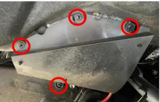
4. Remove the 3 Push Rivets Holding the OEM Felt Wheel Well liner to the body of the vehicle on the Passenger's Side of the vehicle.
