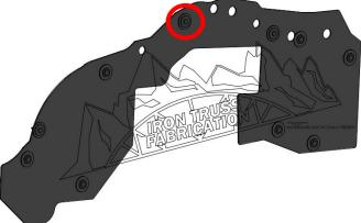
7. Secure the Rear most end of the Front Debris Shield Passenger in place with 3 Plastic Push Rivets **SHORT** and 3 Washers in the locations shown.
