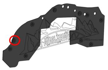
9. Secure the Front most end of the Front Debris Shield Passenger in place <u>UNDER</u> the OEM felt wheel well liner with 1 Plastic Push Rivet <u>LONG</u> and 1 Washer.
