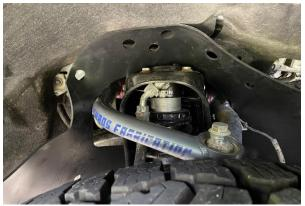
17. Feed the Front most end of the Front Debris Shield Driver between the washer fluid reservoir and the frame/body of the vehicle.
