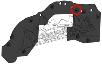
10. Secure the Front most end of the Front Debris Shield Passenger in place with 1 Plastic Push Rivet **SHORT** and 1 Washer.
