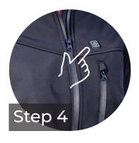
To change heat setting single press the power button to cycle through the 3 heat modes
