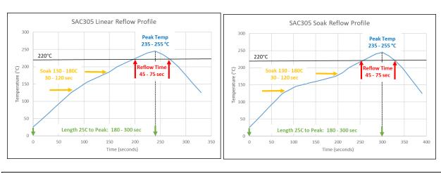
Example reflow profile graphs are shown below. These are a good starting point but they can be modified to fit the product and process. Contact FCT Assembly for assistance with reflow profiling.
