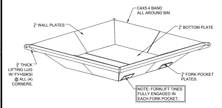
TRAY TARE WEIGHT = 942LB ALLOWABLE LIVE LOAD = 18,000LB ALLOWABLE STRESS BASED ON A FACTOR OF SAFETY =2.0 BASED ON YEILD STRENGTH.
