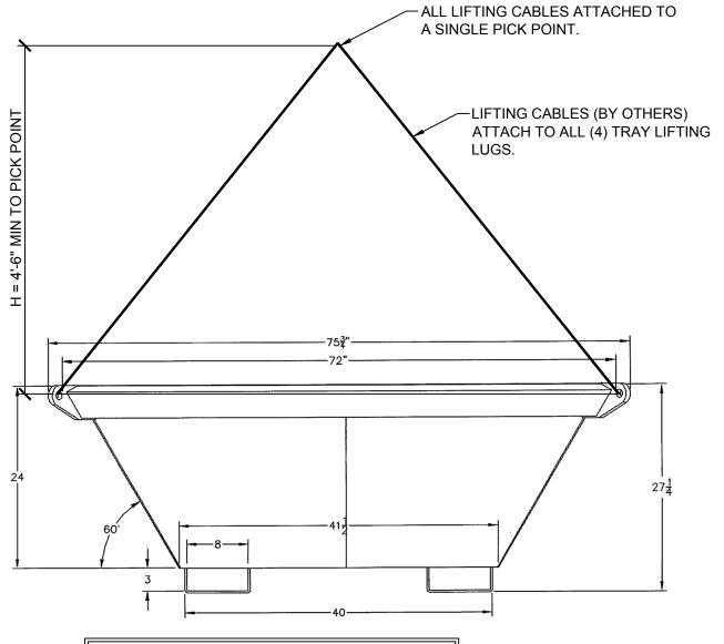
TRAY TARE WEIGHT = 911LB ALLOWABLE LIVE LOAD = 12,500LB ALLOWABLE STRESS BASED ON A FACTOR OF SAFETY =2.0 BASED ON YEILD STRENGTH.
