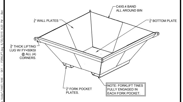
TRAY TARE WEIGHT = 911LB ALLOWABLE LIVE LOAD = 18,000LB ALLOWABLE STRESS BASED ON A FACTOR OF SAFETY =2.0 BASED ON YEILD STRENGTH.
