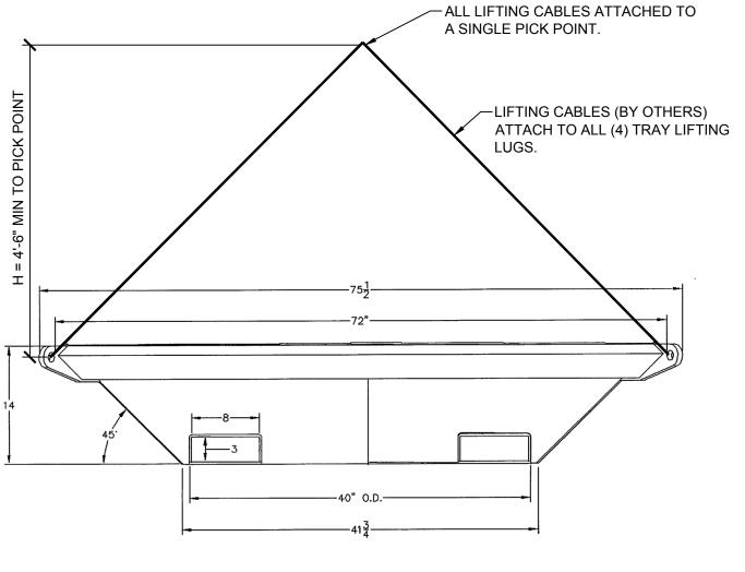
TRAY TARE WEIGHT = 942LB ALLOWABLE LIVE LOAD = 9,600LB ALLOWABLE STRESS BASED ON A FACTOR OF SAFETY =2.0 BASED ON YEILD STRENGTH.
