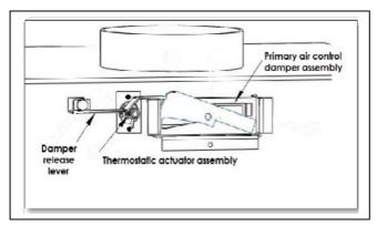
stove. Replace the spring handle. The <u>thermostatic actuator assembly</u> can be replaced by using a 5/16" socket to remove the two screws that hold the assembly. Install the new assembly using the same two screws. The <u>damper release lever</u> can be replaced by removing the  $\frac{1}{2}$ " bolt. When reinstalling the damper be sure it is installed the same as when removed.
