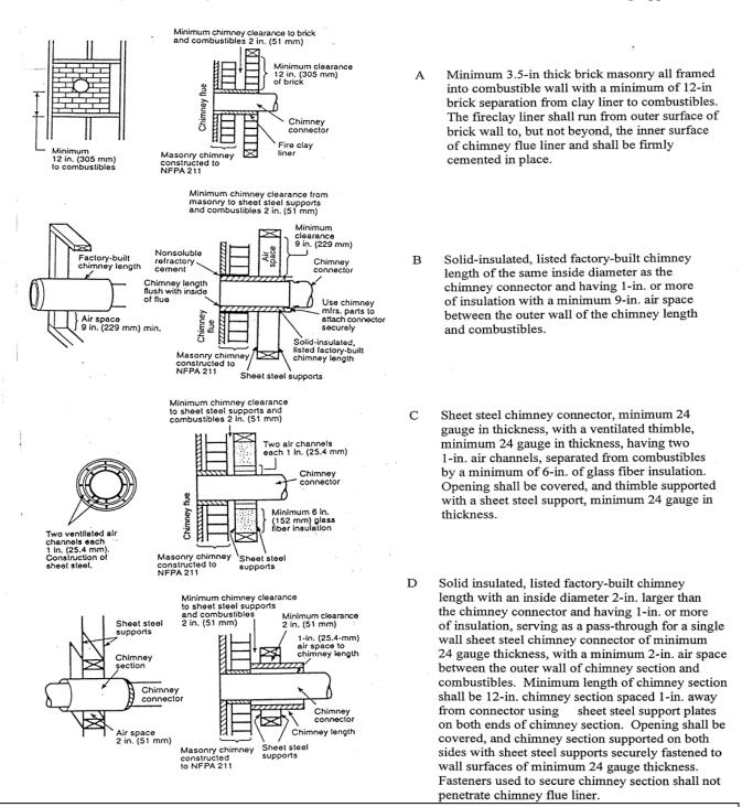
For Canada: A chimney connector shall not pass through an attic, roof space, closet, floor, ceiling, or similar concealed space. Where passage through a wall or partition of combustible construction is desired, the installation shall conform with CAN/CSA-B365.
