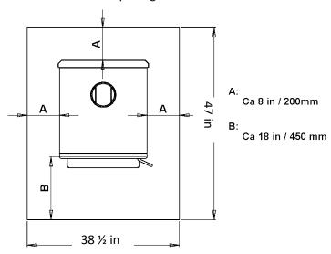
• The spark and ember floor protector must extend 2 in. (50.8 mm.) on either side of any horizontal venting runs and extend directly underneath any vertical venting pipe.
