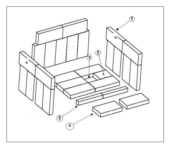
NOTE: The bricks on the sides and rear will need to be installed after delivery \*Top rear bricks on each side may or may not be notched. If notched, order part number AC-SBN1X3.
