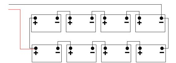
**Note:** Strings are independent, external positive lead is connected to string one, whereas the negative lead is connected to string two.
