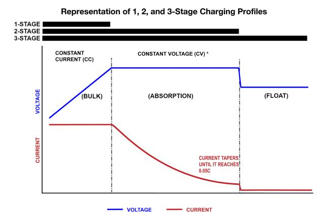
Representation of recommended 2-Stage Constant Current/Constant Voltage (CC/CV) charging. The dotted line represents the transition from CC to CV when the voltage limit is reached. Once the battery reaches the constant voltage limit, the battery is held by the charger at this voltage until the current decreases to 0.05C. At this point the battery is at 100% state-of-charge (SOC). Any current continuing to flow in the float stage is attributable to balancing activity at the BMS.
