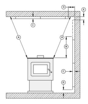
Figure 11: Heat shield clearances
