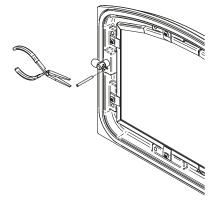
Figure 15: Removing the split pin
