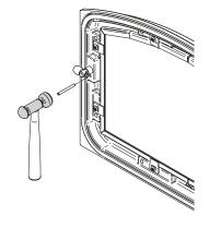
Figure 16: Installing the split pin
