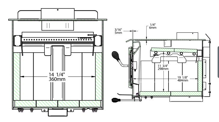
Figure 5: Front View - Combustion Chamber
