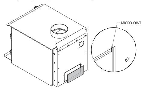
2. Screw the blower (D) in place using the screws (C) included in the installation manual. Screw the thermodisc (A) with the screws (B) supplied with the thermodisc on the back of the stove. Ensure that the blower's power cord is not in contact with any surface of the stove to prevent electrical shock or fire damage. Do not run the power cord beneath the stove.
