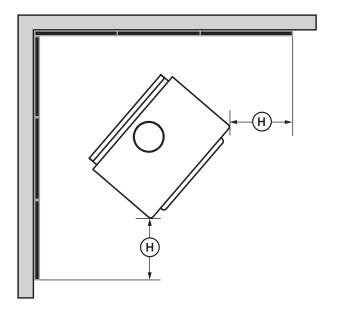
Figure 13: Heat shield clearances
