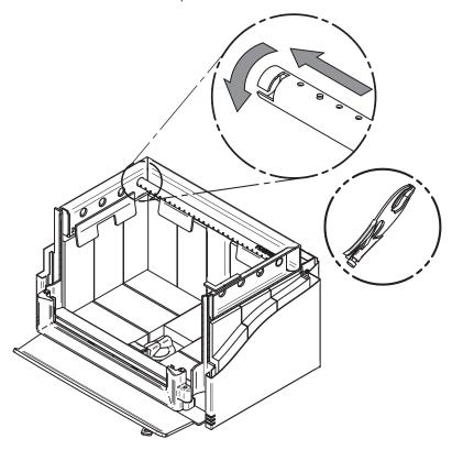
Note that secondary air tubes **(B)** can be replaced without removing the baffle board **(A)** and that all tube are not necessarely identical (look at the part number on the tube).
