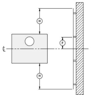
Figure 13: Heat shield clearances
