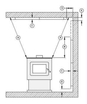
Figure 11: Heat shield clearances
