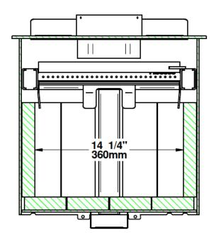
Figure 5: Front View - Combustion Chamber
