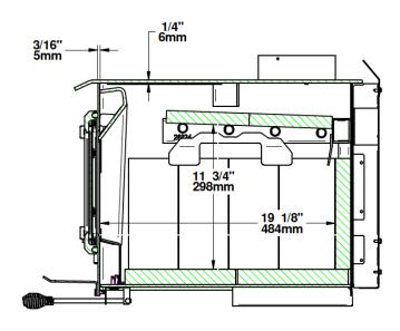
Figure 6: Side View - Combustion Chamber
