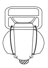
5. Hook the brackets at the bottom of the hooks under the lower edge of your scooter & frame. Hand tighten the nuts until the rack sits firm and even. Then tighten with a wrench.
