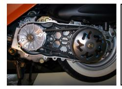
With transmission installed, start scooter and verify smooth, full operation of the transmission.
