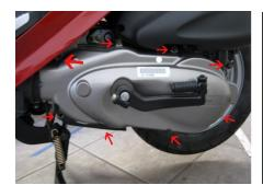
Using your 8mm socket, remove the bolts retaining the transmission cover.
