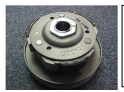
With the rear pulley removed, apply pressure to the clutch and remove 39mm nut.
