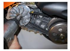
Clean the transmission area with compressed air. Remove the variator and clutch securing nuts with your impact driver or using your strap wrench and 19mm socket.
