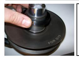
Assemble lower contra spring bearing collar and install onto sliding sheave.
