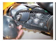
Remove the variator drive face and kick start washer. Remove belt from transmission and inspect. Replace if necessary. (service limit width = 19mm) Slide off variator, drive boss collar and pressure plate.
