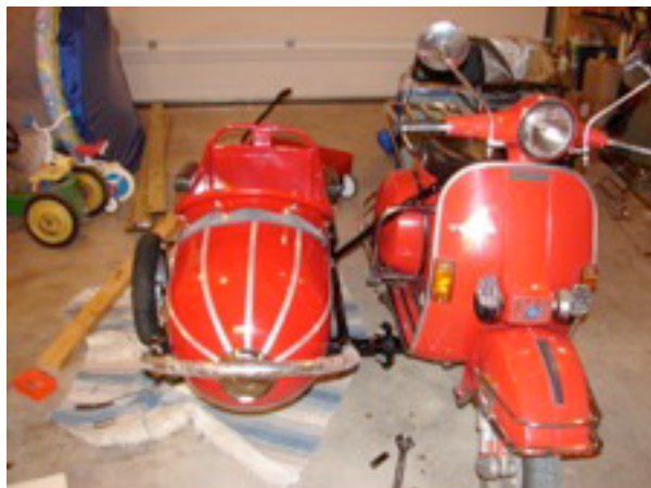
Sidecar chassis attached to frame mount
