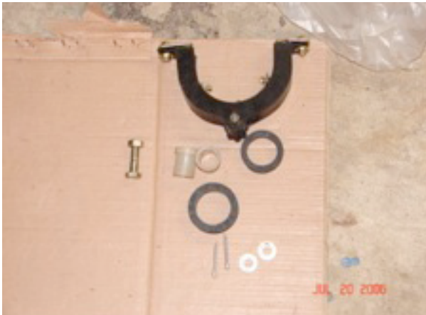
Old style Vespa dampening unit not used for install
