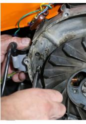
Step 3: Remove the coil assembly.
