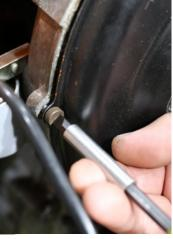
**Step 2:** Remove the remaining fan shroud screws and take off the fan shroud.
