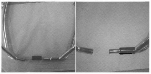
Insert the black sleeve on the rear tube of the cowl protectors.
