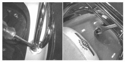
Install the rear rack on the cowl protectors and attach them together. Install the nut to fasten the bracket of the rear rack. You MUST use a spacer under the bracket of the rear rack.
