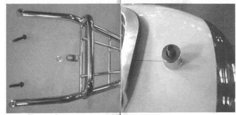
Note the spare parts that come with the Buddy rear rack: 2 longer bolts and 1 spacer. Put the spacer on the rear stud.
