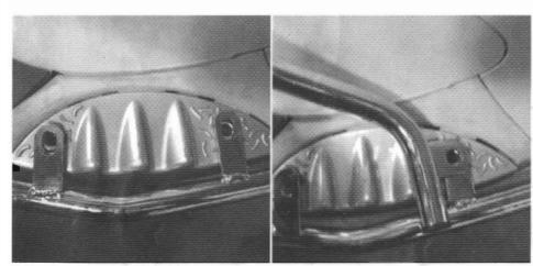
Place the left cowl protector into position as per the picture, then put the footrest on top.
