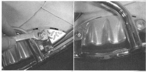
Use the longer bolt to fasten it, but do not tighten it yet. Repeat for the other side.
