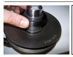
Assemble lower contra spring bearing collar and install onto sliding sheave.
