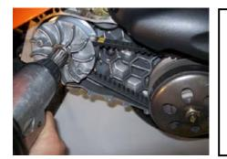
Clean the transmission area with compressed air.
