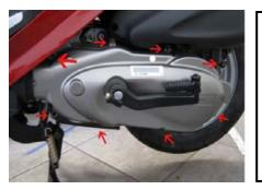
Remove the bolts retaining the transmission cover.
