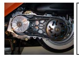
With transmission installed, start scooter and verify smooth, full operation of the transmission.
