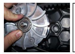
Place supplied roller weights into variator and install backing plate.
