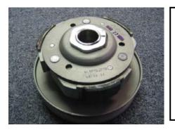
With the rear pulley removed, apply pressure to the clutch and remove nut.
