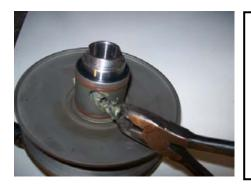
Remove guide pins using pliers. Use caution as marring or gouging the pins will cause excessive wear.
