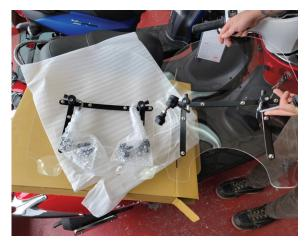
**Step 5:** Rotate Hardware to the outward position. (Opposite to how the hardware is packed)
