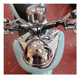
**Step 2:** Use 17mm wrench to loosen headlight bolt, and lower headlight.
