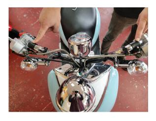
**Step 4:** Position the inner clamp gaskets on the handlebars and flush to the master cylinder(s)
