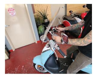
**Step 12:** Use 13mm wrench and 6mm hex to tighten adjustment nuts once screen angle is set.
