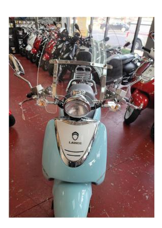
**Step 13:** Fully tighten 2nd set of screws on the bar clamps.
