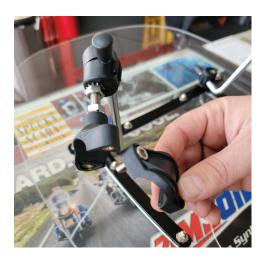
**Step 1:** Remove from Box. Use 5mm hex to unscrew half of each bar mount.
