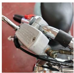
**Step 3:** Use 6mm hex to loosen and lower master cylinders (1 master cylinder on Cali 50 and 125. 2 for Cali 200)
