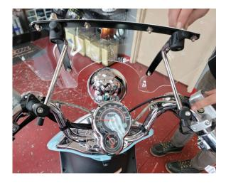
**Step 6:** Line up bar mount halves on the inner clamp gaskets.
