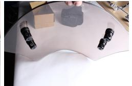
**Step 10:** Install hardware on windshield and align strut mount holes
