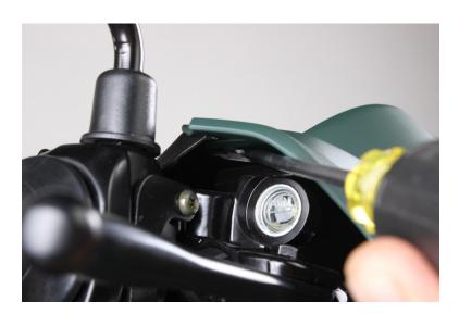
**Step 3:**Carefully release clip with a long flat screwdriver.
