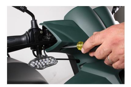
**Step 2:**Remove screw with a #2 Phillips screwdriver.
