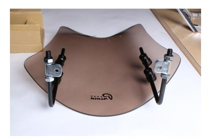
**Step 11:**Loosen Allen set screws on mounts and slide struts through mounts
