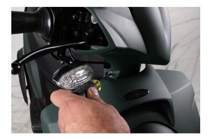
**Step 1:**Remove screw with a #2 Phillips screwdriver.
