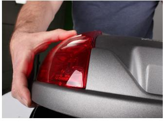
Step 11: Re-install reflector and lens sets.
