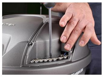
**Step 8:**Screw down LED strips to preformed location.
