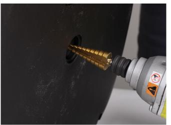
Step 2: Drill hole in the base center. A dremel is very helpful in order to clean up hole to the proper size. Make sure to be very careful not to drill/ dremel hole too large.
