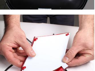
**Step 10:** Tear off serrated portion of reflector to accommodate LED strips.
