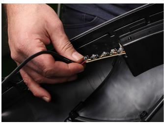
Step 7: Fit LED strips through the access slot, right side and left side accordingly.
