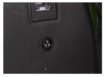
**Step 3:** Feed LED strips through the hole and set inside topcase.
