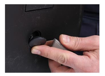
Step 1: Pull off plug located on the bottom of your K-Max 30 Liter Topcase.
