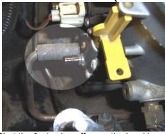
4. Shut the fuel valve off once the bowl has drained. Pull the drain tube connector off of the valve. The nipple that the hose connects to is plastic so be careful not to force it up or down, just pull straight towards the rear of the block. There are four screws holding the valve assembly to the bowl. (pre-99 OBS 7.3L have only 2 screws)
