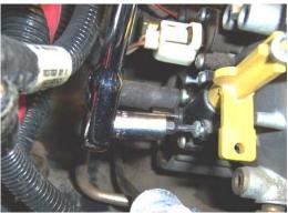
**5.** The screws require a #20 torx bit. Using a ¼" ratchet and socket to hold the torx bit, remove all four screws. It will be helpful to keep a magnetic pick up tool or grab tool handy in case you drop your wrench in the engine block valley.
