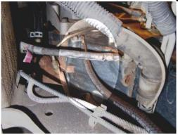
1. Locate the drain tube that comes from the fuel bowl. It is under the passenger side valve cover, directly below the A/C compressor. Slide a 30" piece of hose over the tube and route it to the shop floor. You should place a catch can under the hose so when the fuel bowl is drained, the fuel will be contained in the catch can.
