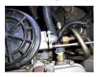
3. With a #25 torx screwdriver or bit, remove the 2 bolts from the FPR cap evenly. If you remove one completely and then the other, the pressure from the spring can put undue strain on the bolt ear of the remaining bolt. Pull the cap straight off the spring and remove it from the brass regulator piston seat.
