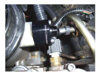
IMPORTANT: If replacing the cap due to breakage of the factory cap and you cut and re-flared the return line, the flare MUST be small enough so the flare fits inside the threaded nipple on the regulator cap. If the flare is too large, the compression sleeve will not seal the line to the housing.
