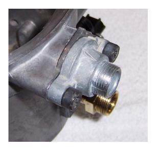
8. With a #25 torx screwdriver or bit, remove the 2 bolts from the FPR cap evenly. If you remove one completely and then the other, the pressure from the spring can put undue strain on the bolt ear of the remaining bolt. Pull the cap straight off the spring and remove it from the brass regulator piston seat.
