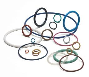
The thermal stability of fluorosilicones accomodate all automotive fuel applications and almost all aerospace applications. The elastomersare used for their outstanding low temperature properties, having a functional temperature ranging from -100°F to +350°F (-73°C to +177°C). Because fluorosilione o-ring elastomers have unmatched low temperature performance and good hydrocarbon compatibility, they have become the standard seal material in numerous applications.
