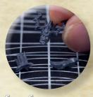
STEP 6A Remove all three parts from the sprue and clean excess flash.
