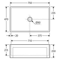
Please note: Butler sink measurements shown are a guide only. For installation, measurements must be taken from physical product received.
