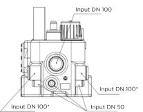
\*This entrance must be directed at a height of 250 mm above the ground level directly after the lifting station.
