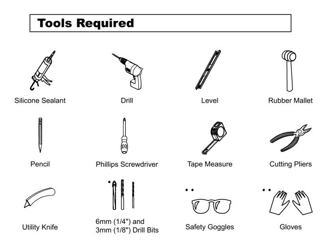
\* Use the correct type of drill bit for the material being drilled, with 6mm required for anchor fixing and 3mm used for screwing directly into the wall studs.
