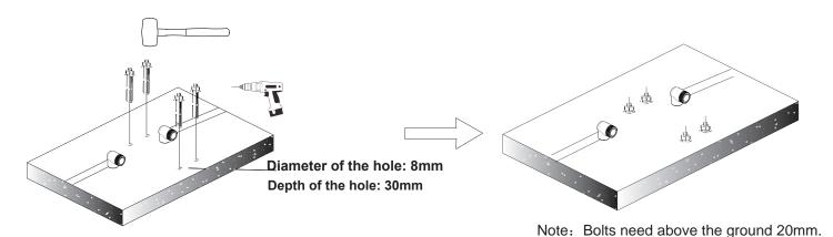
4. Drill - knock in expansion bolt - pre-tight - remove nut and washer
