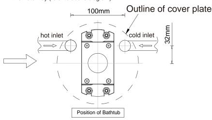
3. Place the mounting seat in the middle of the two water inlets, mark the holes of bolts.
