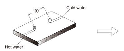
1. Determine the position of floor mounted bath mixer, spout should be in the range of bathtub. Pre-embed the waterway (refer to above diagram).
