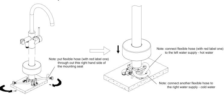
1. Fix the mounting seat then tighten bolts firmly by using a spanner.
