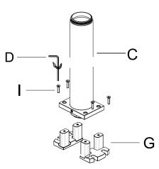
2. Using screws to fasten standpipe C and mounting seat G.
