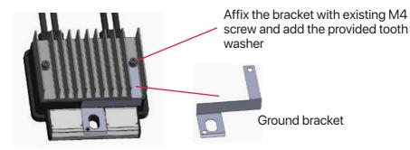
Once the assembly is installed to the PV module frame, drill a 4mm diameter hole through the metal PV module frame in line with the ground hole in the grounding bracket, as per the diagram below. Secure the bracket with a M3.5 self-tapping screw and a M3.5 tooth washer or equivalents. Note that the self tapping screw and tooth washer are not provided.
