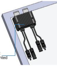
Recommended orientation of the Enteligent NMax M900A1 on module frame after mounted as shown (heatsink face outwards). • Use bracket clip mount to module frame, just simply insert the clip up to the end into the frame in the desired location.
