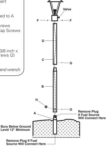
7. When installation is complete, open gas supply valve and test all gas connections with soapy water before lighting. Do not use a match or open flame to check for leaks. Correct all leaks and test with soapy water before lighting.
