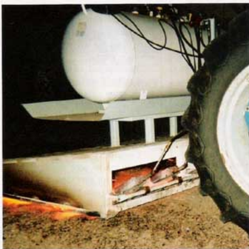
A standard 120-gal. fuel tank is recommended to supply the sterilizer's six liquid propane torches that maintain the heat at a minimum of 1400°F. Photo courtesy of Welch Gas.
