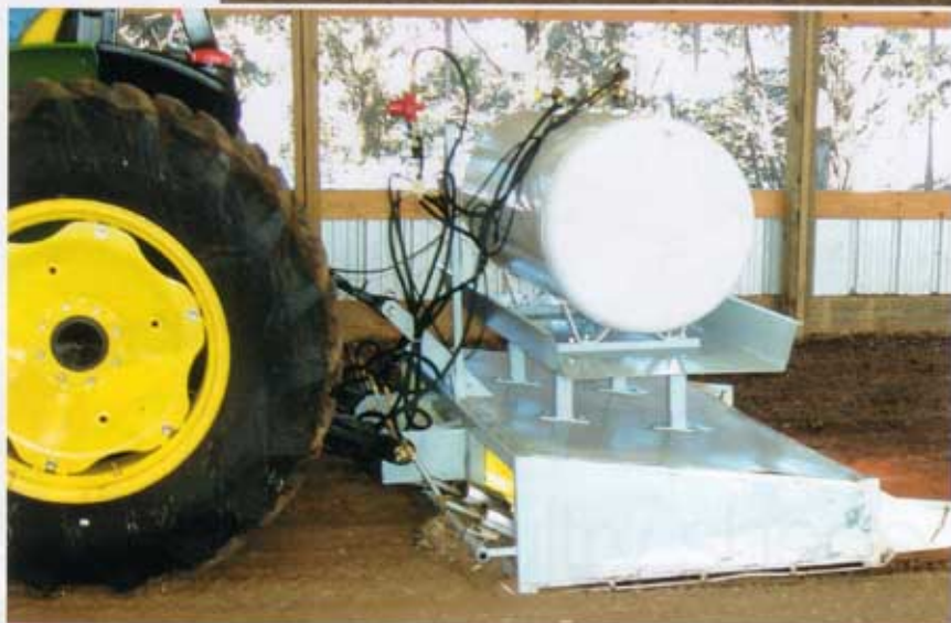
Top: Temperatures reach around 750 degrees C under the steel hood. Above left: Red Dragon Flame Sterilizer uses standard 120 (US) gallon tank. Above: Red Dragon effectively kills pathogens in poultry sheds.
