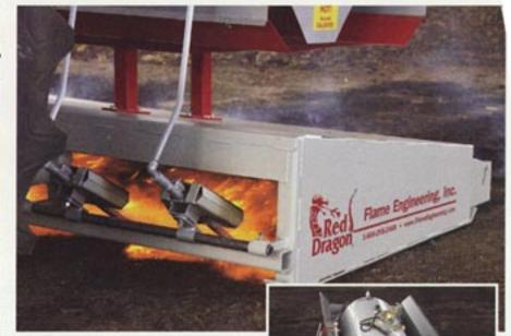
PROPANE BURNERS heat the ground to 2,000 degrees F beneath the Red Dragon's stainless-steel hood. Researchers say the trial by fire kills viruses and bacteria with no residues.
