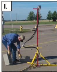
7. Arrange the tower so that the tripod leg with the hose bracket is pointing toward the tank being evacuated. Weight the tripod legs with cinder blocks or sand bags if the unit is to be operated on pavement. If the unit is to be operated on dirt or grass, stake each tripod leg down using the leg stakes included with the unit. (see photo I)
