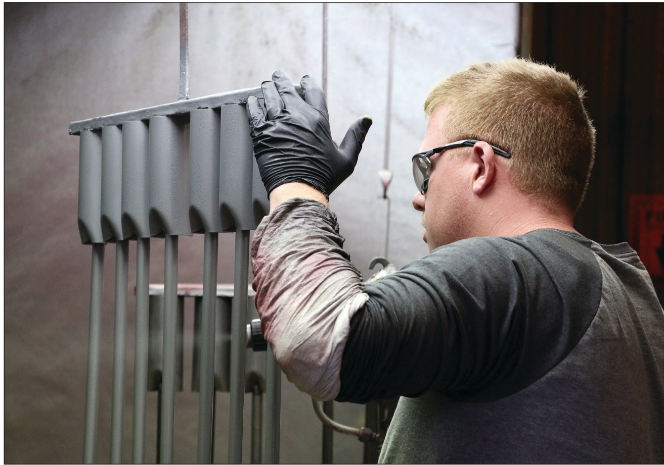
Darren Volkel paints a row of torch bells in the painting room at Flame Engineering in La Crosse.
