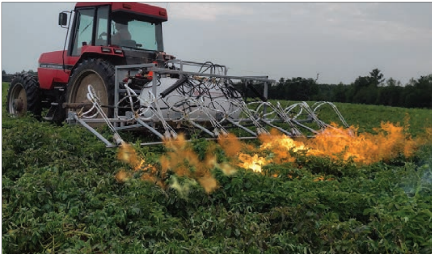
The patented liquid spray flaming process in action.
