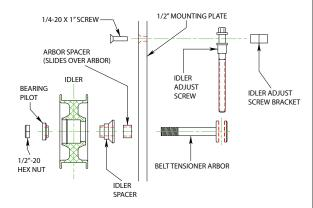
Fig. 7-b (10-Rib Belt Tensioner Assembly - Side View)
