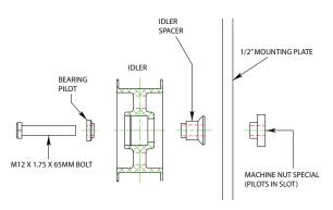
Fig. 7-c (Cog Belt Tensioner Assembly - Side View)
