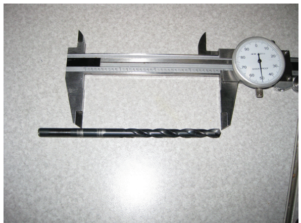
Fig. 1-c: Mark Drill Bit Depth To 2.27"
