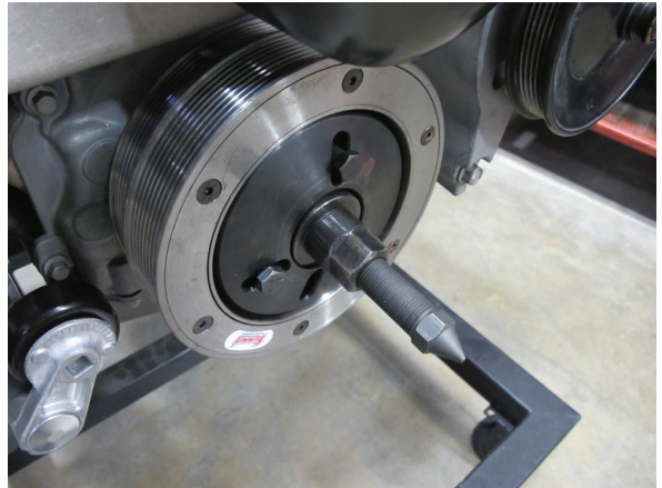
Fig. 1-b: Install Provided Damper
