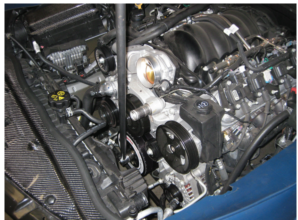
Fig. 1-f: Install & Torque Damper Bolt
