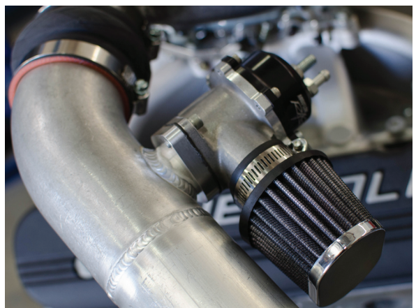
Fig. 4-i: Install Bypass Valve
