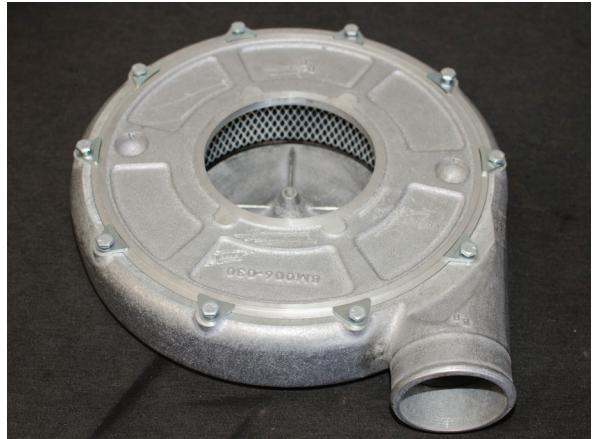
Fig. 4-b: Re-install Carburetor Hat Base
