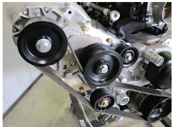
Fig. 3-f: Install 10-Rib Drive Belt
