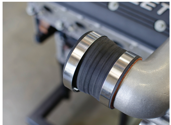
Fig. 4-f: Install 3.00"-2.75" Reducer Sleeve
