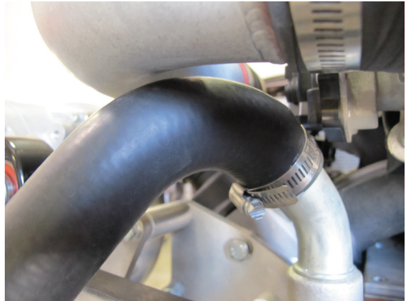
Fig. 5-d: Install Modified Coolant Hose Elbow
