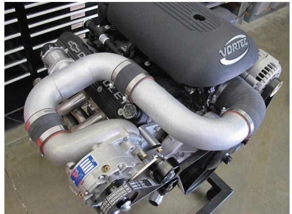
Fig. 4-d: Install Discharge Tube B
