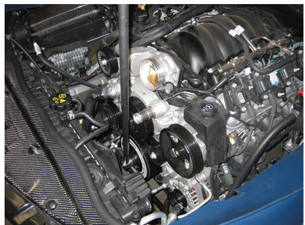
Fig. 1-f: Install & Torque Damper Bolt
